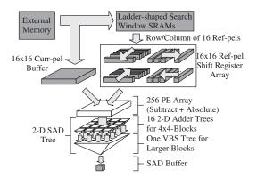
Fig. 6. Architecture of integer motion estimation. The dark gray parts are the memory units. The light gray parts are the data flows. The white parts are the processing units.
