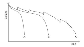
Fig. 1. Battery discharging effects of three kinds of video encoders. A is a general encoder. B is a low-power encoder with 50% power consumption as compared to A. C is a low-power and power-aware encoder.
