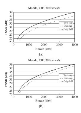
Fig. 8. Rate-distortion performance of the proposed one-pass FME algorithm. The solid, dashed, and dotted lines show the performance of the two-step algorithm in the reference software, the proposed one-pass algorithm, and the algorithm with only half-pixel refinement.
