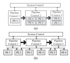
Fig. 11. Illustration of two types of control systems. (a) Conventional twolayer control system. Processing engines can be operated in only one pipeline stage and (b) proposed three-layer control system. Processing engines are flexibly operated in different pipeline stages.
