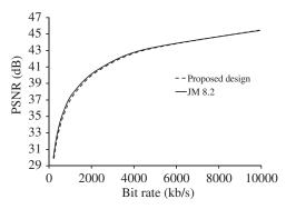
Fig. 14. Rate-distortion curve of the proposed H.264/AVC encoder for D1  $(720 \times 480)$  30 frames/s *Soccer* sequence. Only 1 reference frame is used in this simulation.
