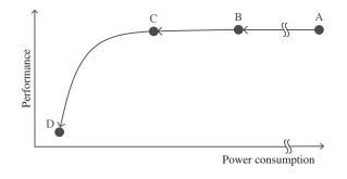
Fig. 2. Power-performance curve of different real-time video encoding systems. Point **A** is a general encoder without optimization. Point **B** is an architecture-optimized encoder. Point **C** is an encoder with algorithmic and architectural co-optimization. Point **D** is an ultra low-power encoder with minimized computation but the worst coding performance.
