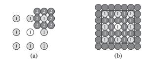
Fig. 7. Illustration of fractional motion estimation algorithm. The white circles are the best integer-pixel candidates. The light gray circles are the half-pixel candidates. The dark gray circles are the quarter-pixel candidates. The circles labeled "1" and "2" are the candidates refined in the first and second passes, respectively. (a) Conventional two-step algorithm and (b) proposed one-pass algorithm. The 25 candidates insides the dark square are processed in parallel.
