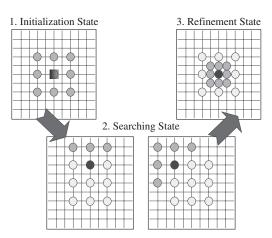
Fig. 3. Searching flow of four-step search. In the initialization state,  $3 \times 3$  candidates with the step of two pixels are searched. In the searching state, the searching pattern moves according to the best matching candidate in the previous iteration. Finally, if the best matched candidate is the central point, the refinement is performed around the neighboring eight candidates.
