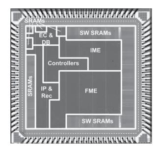
Fig. 13. Chip photo of the proposed H.264/AVC encoder.
