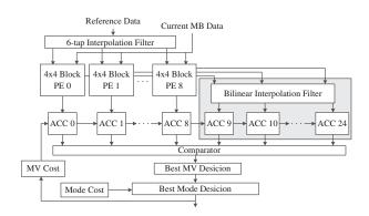
Fig. 9. Architecture of fractional motion estimation. The processing engines on the left side are used to generate the matching costs of integer-pixel and half-pixel candidates. The transformed residues are reused to generate the matching costs of quarter-pixel candidates with the processing engines inside the light gray box on the right side. Then, the 25 matching costs are compared to find the best MV.
