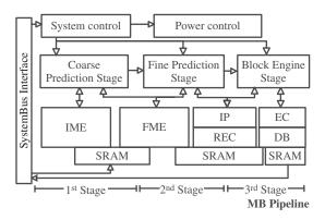
Fig. 12. Proposed system architecture for the H.264/AVC encoder. The three-layer control system is adopted to improve system flexibility, including the system control, the pipeline control, and the PE control. There are three MB-pipeline stags comprising "Coarse Prediction," "Fine Prediction," and "Block Engine" stages. "Power control" is used to online monitor the states of processing engines and stage controls. Once they enter the idle state, the clock sources will be gated for power saving.
