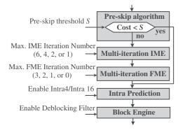
Fig. 10. Illustration of the parameterized power-scalable H.264/AVC encoder. "IME Iteration Number" is defined as the number of initial candidates for the proposed parallel-VBS-FSS algorithm. "FME Iteration Number" is defined as the number of refined inter-modes for the proposed advanced mode predecision algorithm. More than 128 configurations can be provided in this system.
